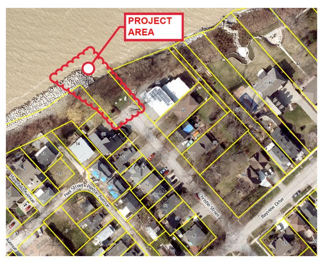
The proposed construction project includes: installation of pedestrian access to Lake Ontario at the termination of Christie Street, including a concrete pathway, steel stairs, concrete stairs, bench & bike rake and site restoration.
