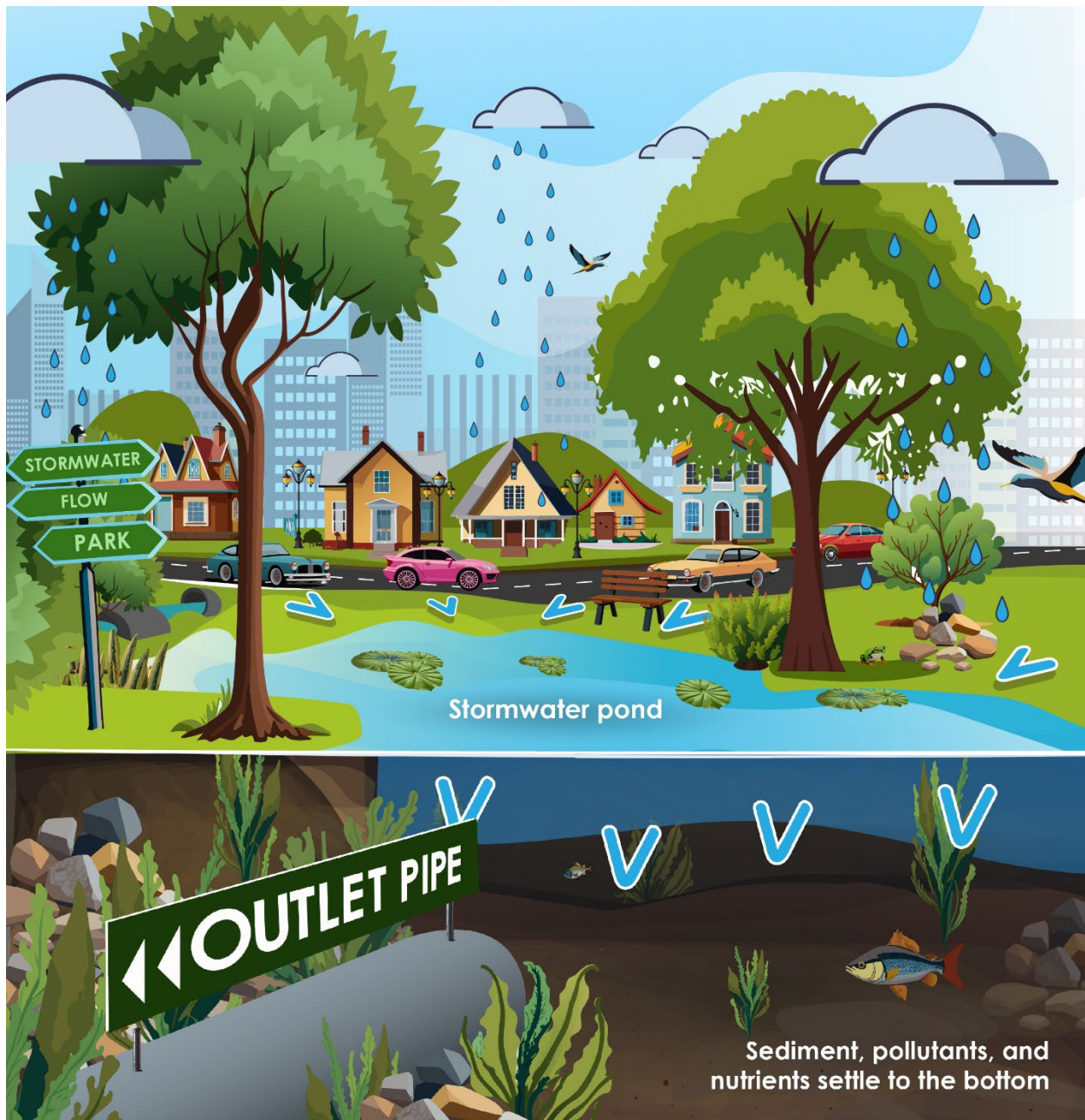
Figure 4: Typical Stormwater Pond
